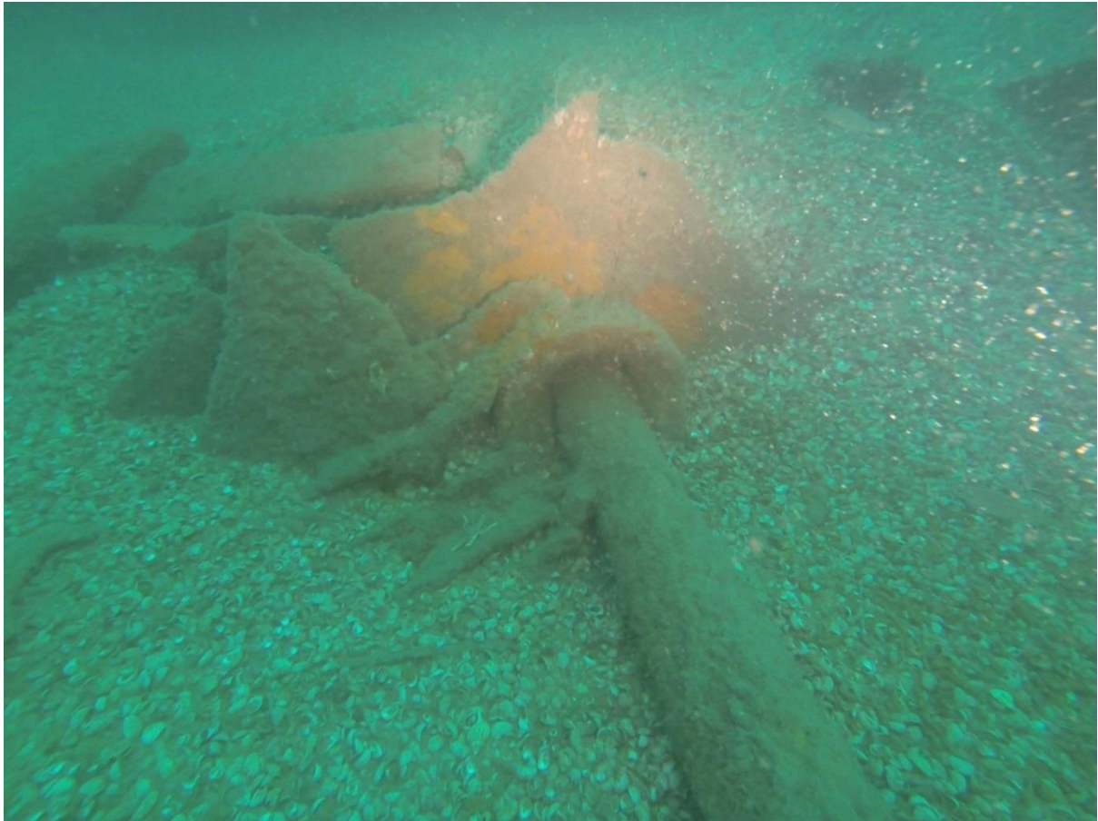
Photo 14, Opposite end of the displaced prop shaft seen in Photo 12. Note the ragged edges to the bulkhead housing a bearing.
