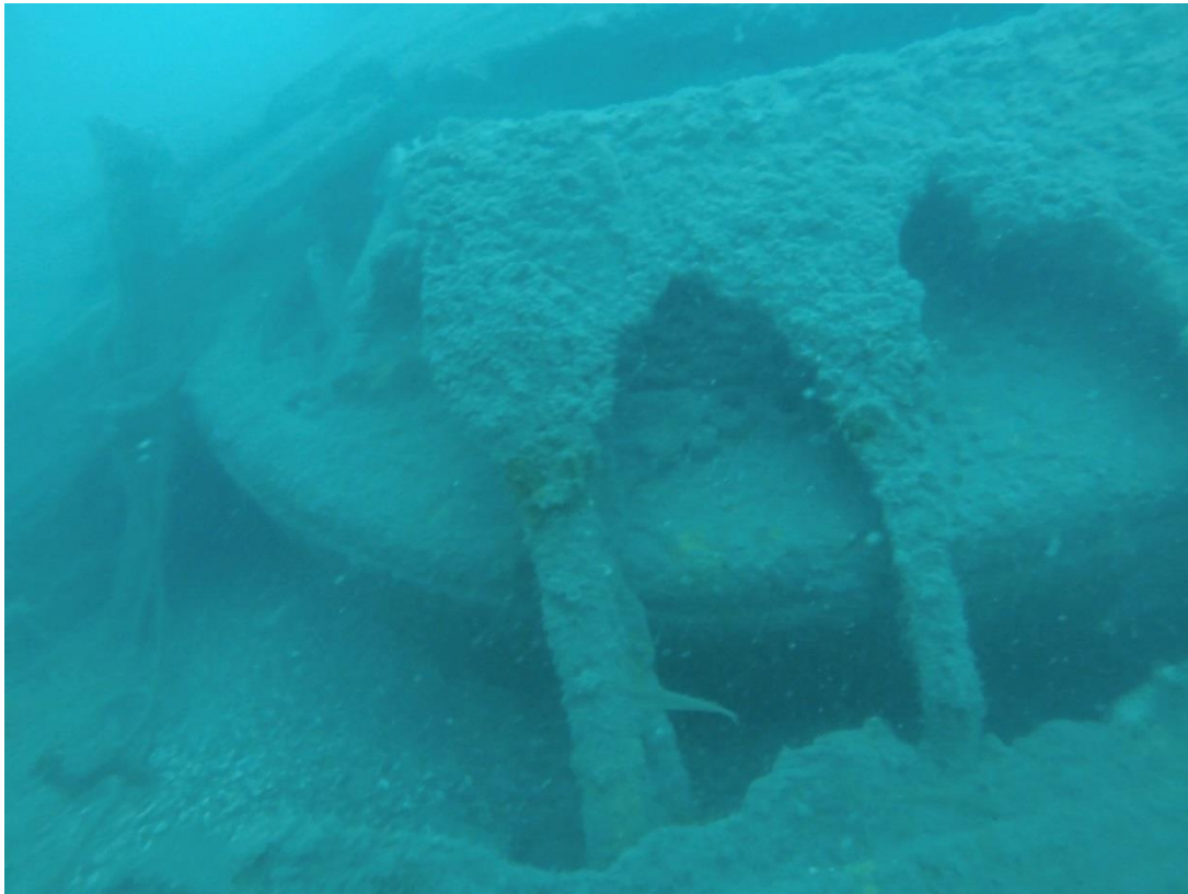
Photo 19, Boiler lying on its aft end, with exposed fire tubes and overlain by the hull ribs.
