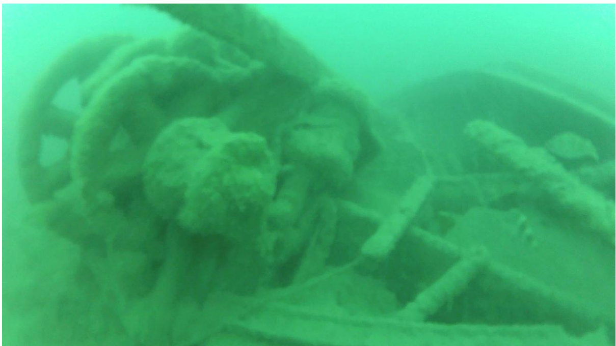
Photo 15, Steam anchor winch lying upside down.
